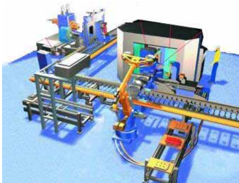
Figure 8. Segment flexible technological structure where fixture manipulation is done by robot
