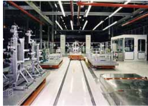
Figure 9. Segment flexible technological structure where fixture manipulation is done by rail guided vehicle
